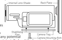
Make certain that the lens shade has been threaded completely into the camera to avoid any potential clearance or sealing problems when the camera is installed and the housing is sealed.
